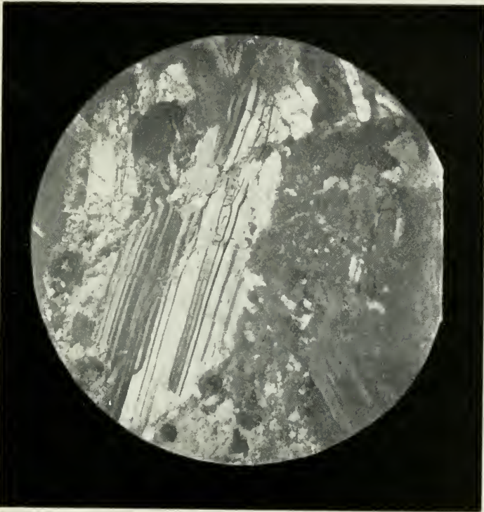
MICROPHOTOGRAPH, ILLUSTRATING FAULTING OF FELSPARS.
